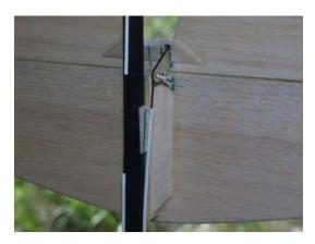
• For the rudder make a 3<sup>-5</sup>mm L bend at the end of the wire and insert into the control horns's *middle* hole
