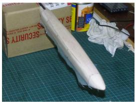
• After the first coat has dried partially (approximately 3 hours for a lot of varnishes) cut off the excess cloth using a sharp No.11 blade
