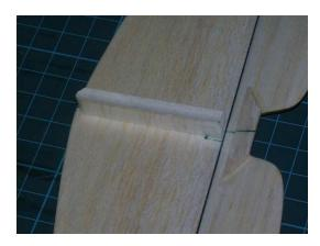
• Due to the stresses involed on the tail feathers and the thin wood they're made of (1.5mm), it's important that the load between the boom and the horizontal stabilizer is spread out. To do this we add some 6x6mm triangular stock on either side of the exiting interface. Remember to cut away the tape hinge where required.
