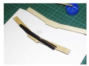
Clamp together the dihedral brace sandwich, don't worry if some CF tow protrudes from the assembly, this can be trimmed off • later.
