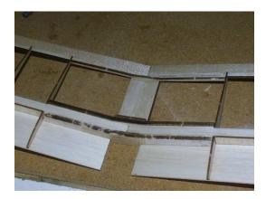
• When the dihedral brace bond is dry you can proceed to glue the trailing edges to the TE dihedral brace (ideally they will already be well lined up with the brace).
