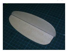
• Hold the two halves down flat and apply a second piece of 12mm clear tape to the opposite side
