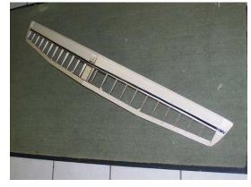
• Check that the wing's LE is straight by placing the wing LE down onto a flat surface. The wing should sit very flat to the surface.
