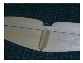
• Before attempting to bond the boom to the tail feathers it's important to lightly roughen up the boom using some 200 grit or finer sand paper up to 135mm from the end of the boom. Once you have done this, wash the boom under water and wipe dry, the boom should appear slightly more matt in appearance where the sandpaper was applied
