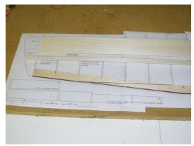
• Trim away a portion of the bottom D box sheeting so that the dihedral braces and wing mount block can fit in when the two wing halves are finally assembled.
