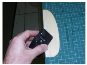
• Bevel the join edge of the rudder using a balsa plane (or other tool) to approximately 45 degrees
