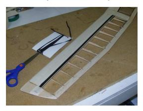
• Flatten out and groom the CF tow until it is approximately 10~12mm wide, we need to get the CF tow this wide so that it remains as flat as possible against the D-box sheeting
