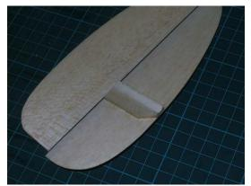
• When bonding the vertical stabilizer to the boom, it's very important that it is set up at 90 degrees to the existing horizontal stabilizer. There are many different ways that this can be done. We have used some right angle aluminium channelling to which we clamped on both the existing horizontal stabilizer and then the vertical stabilizer.
