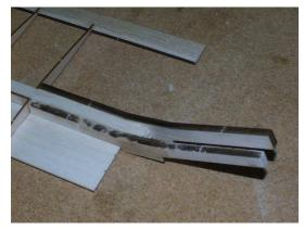
• Obtain and glue a single 30 x 15 x 3.2mm brace doubler and glue it to the rear dihedral brace. This is a spacer used to add yet more strength to the dihedral join and distribute the load.
