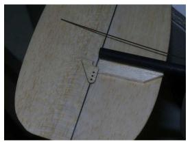
• Mark the location of the base of the control horn with a pen, this is where we will cut out a slot that the control horn will be placed. The control horn must be just slightly lower than the boom so as to allow for the control wire to slide freely without binding when the control horn is pulled inwards towards the boom.
