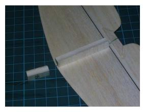
• Mark the width of the interface on the tape hinge. We do this so we know where to cut away the tape. If we don't cut away the tape, when we bond the interface to the horizontal stab it won't stick in that area causing a potential weakness.
